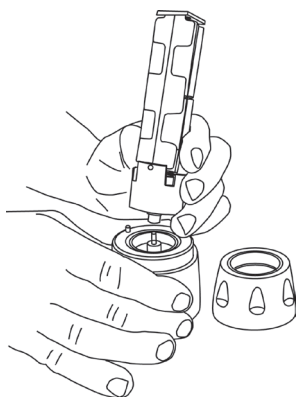
Drawing 8 - Correct insertion of the battery casing
